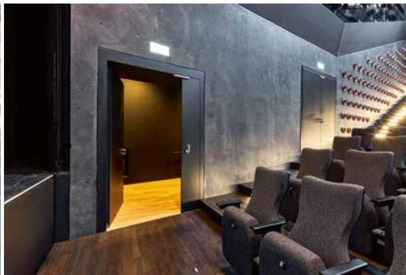
The floor between the stage and second row of seats can be lowered if required. The space produced can then be used as an orchestra pit.
